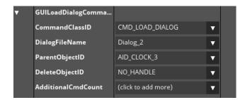
This command loads a new dialog and places it into the specified CompositeObject. Additionally a given object can be deleted.
