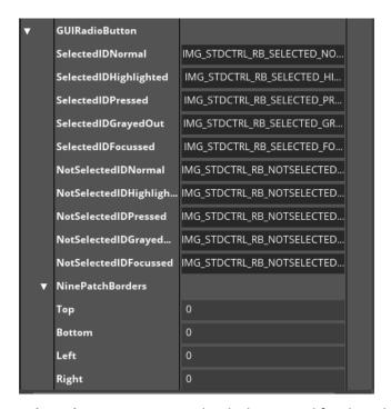
**SelectedImageIDs**: Image-ids which are used for the selected-state according to the state of the object
