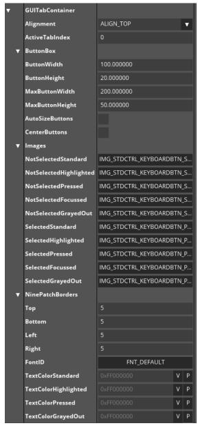
**Alignment:** this specifies the placement of the button-box. It can be ALIGN\_TOP, ALIGN\_BOTTOM, ALIGN\_LEFT or ALIGN\_RIGHT
