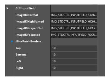
ImageIDNormal/ImageIDHighlighted/ImageIDGrayedOut/ImageIDFocussed: image ids which will be used as the background of the input-field according to the current state of the object.
