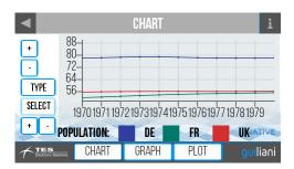
This sub-dialog contains a *Chart* which can display discrete values of multiple data-series like in some spreadsheet-program. The buttons on the left are all attached to *CallAPI* and control the zoom and type of the *Chart*.
