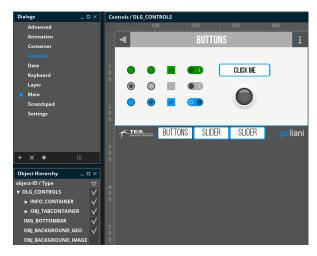
So we created sub-pages (red) containing a small part of the controls which can be dynamically shown by the buttons on the bottom of the screen. Each of these sub-pages is a *TabItem* inside the Client-area of a *TabContainer*.
