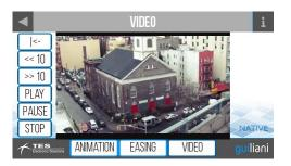
This sub-dialog shows the video-file, which is randomly picked when the dialog is loaded and additional buttons which are used to control the video, e.g. play, stop, rewind. All the buttons are attached to *CallAPI*-commands which execute the various actions.
