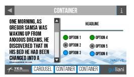
In this sub-dialog the screen is divided into three parts with a large *TextField* which can be swiped, a static *TextField* and several *RadioButtons*. Each of these parts can be resized by dragging the splitter-handle.
