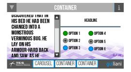
In this sub-dialog the screen is divided into three parts with a large *TextField* which can be swiped, a static *TextField* and several *RadioButtons*. Each of these parts can be resized by dragging the splitter-handle.
