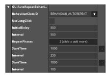
The *AutoRepeat*-behaviour can be used to execute a command attached to the control several times in a specific period.
