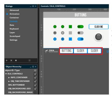
So we created sub-pages (red) containing a small part of the controls which can be dynamically shown by the buttons on the bottom of the screen. Each of these sub-pages is a *TabItem* inside the Client-area of a *TabContainer*.
