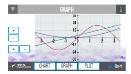
This sub-dialog contains a *Graph* which displays three different functions. The buttons can be used to zoom in or out the x- and y-axis via *CallAPI*.
