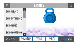
Here we have a list of the various easing-types available in Guiliani for any dynamic visuals, i.e. animations and an object which will move down towards the bottom-bar using the selected easing.
