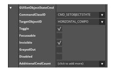
The groups on the left and on the right have a *CheckBox* above them which uses *SetObjectState* to control the visibility of the containers surrounding the controls below.
