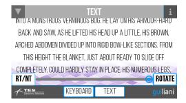
This dialog is very simple as it only shows a large text – either as a *TextField* or as a *RichTextField* – and a Slider which controls the width of the shown text.
