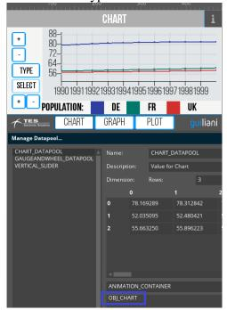
The *Chart* is connected via a *DataPool*-entry. Since *DataPool*-entries can have not only one value, but also two-dimensional arrays of value, this *DataPool*-entry has multiple values.
