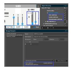
The group on the right, consisting of a *TextField*, a *ProgressBar* and a *Slider*, has a connection via a *DataPool*-entry.
