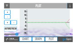
This sub-dialog shows a *Plot* which displays dynamic data simulated by the application. The buttons are used to zoom in or out the x- and y-axis via CallAPI. The button "*AutoRefresh*" will toggle the auto-refresh for the *Plot* and the slider the period of the refresh.
